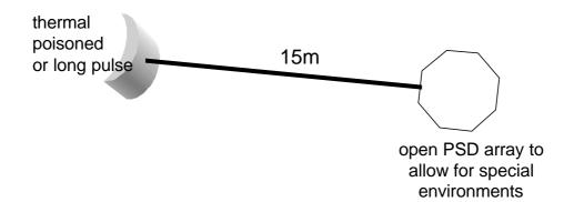
Generic type:D10 (ILL), 6T2 (Saclay), TAS in elastic modeWavelengths used:0.5-5 ÅModerator Type:thermal, decoupled
