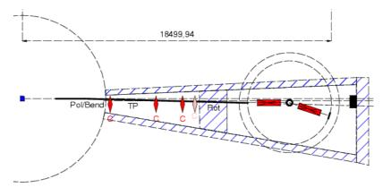
**Generic type:** Wavelengths used: Moderator type: IN11 ; Fourier method -> S(Q,t)0.2 nm <  $\lambda$  < 2 nm cold coupled hydrogen
