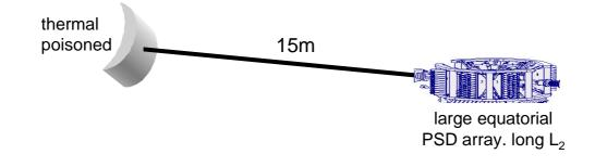
Generic type:D9, D10 (ILL); SXD (ISIS), SCD (IPNS)Wavelengths used:0.25-2 ÅModerator Type:thermal, poisoned, decoupled (dt~10µs)
