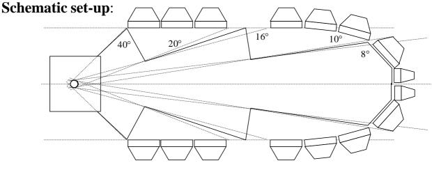
Generic type. Wavelengths used: Moderator Type: Q-range: SANDALS/GEM TOF diffractometer 0.05 Å – 5.0 Å water (50Hz) – preferred 0.01 Å<sup>-1</sup> < Q < 60 Å<sup>-1</sup>
