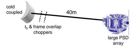
Generic type:LADI, D19 (ILL); PX-station (LANSCE)Wavelengths used:1.8-5 ÅModerator Type:cold, coupled (but 3-5 x gain if 130K mod.)
