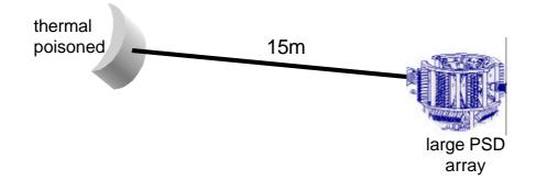
Generic type.D9 (ILL); SXD (ISIS)Wavelengths used:0.5-5 ÅModerator Type:thermal, poisoned, decoupled (option of 130K)
