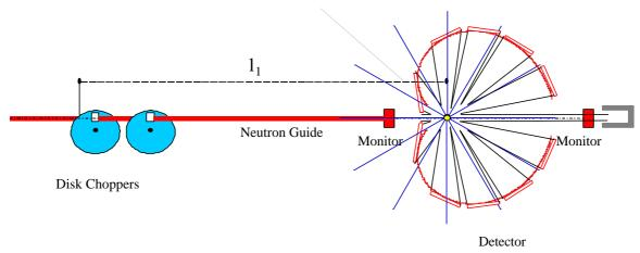
**Generic type:** Medium-resolution powder diffractometer crystallographic applications
