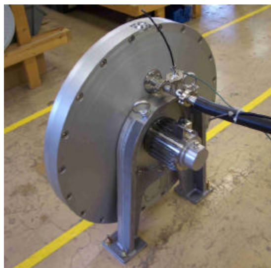
Fig. 5 A CFRP-Disk (upper panel) and a Housing (lower panel) of a Prototype High-Speed Disk-Chopper of CNMCS.
