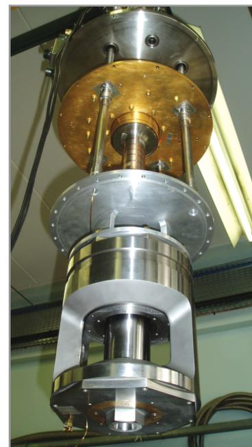
Internal view of the 3K cryogen-free cryostat hosting the Paris-Edinburg pressure cell.
